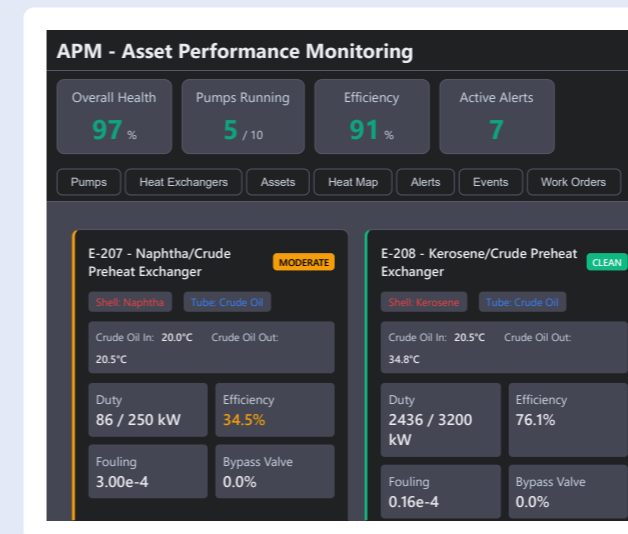
HEAT-EXCHANGER HEALTH CARD — DUTY, FOULING, CLEANING RECOMMENDATION, TUBE/SHELL TEMPERATURES AND U-COEFFICIENT DEVIATION
